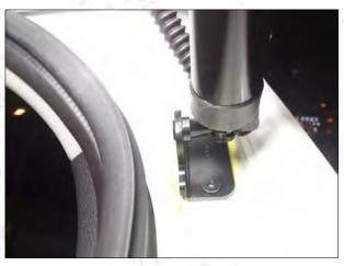
5.Remove the original car right lower bracket. Install our right lower brackt and fix it with our screws. Then install our brace rod.
