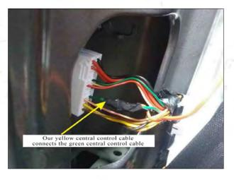
12. Remove the trim panel from the main driving side and find the central control.
