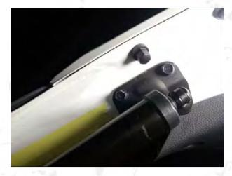
2.Remove the original brace rod. Use the original upper bracket to install our brace rod (Note: Need someone to hole the door)
