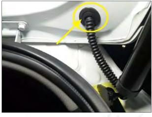
6.Remove the original car rubber plug. The Hall line passes through the hole and put the rubber plug on it.
