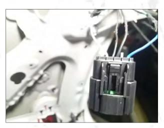
14. Find this socket at the rear door lock position and unplug it, insert it into our three-way adapter socket. And insert the other end of the three-way plug into the position of the door lock.
