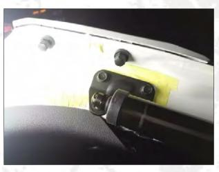
4.Install our brace rod with the original car upper right bracket.
