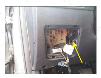
7.From here, the Hall line runs through the waterproof rubber plug, and the cable is routed to the central control box, and the control box is inserted as shown in the figure.
