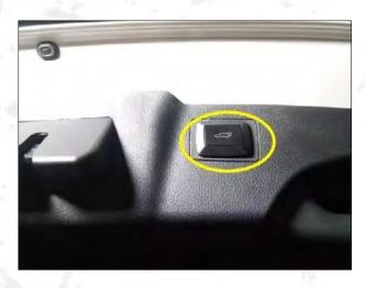
16.Punch hole in the original tailgate trim panel and install our tailgate switch button.
