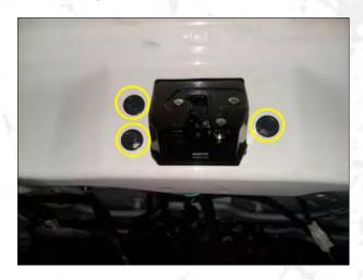
15.Remove the original door lock, install our top electric suctio lock and fix it with the original car screws.
